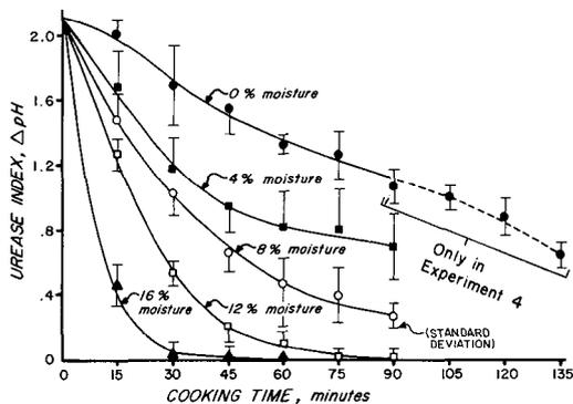
FIG. 1. Composite data of Experiments 3 and 4 showing the effect of moisture and cooking time on soybean meal urease index.
