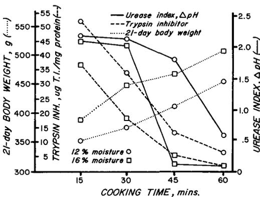
FIG. 4. Comparison of urease and trypsin inhibitor as indicators of soybean meal processing adequacy.
