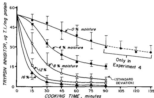
FIG. 2. Composite data of Experiments 3 and 4 showing the effect of moisture and cooking time on soybean meal trypsin inhibitor contents.
